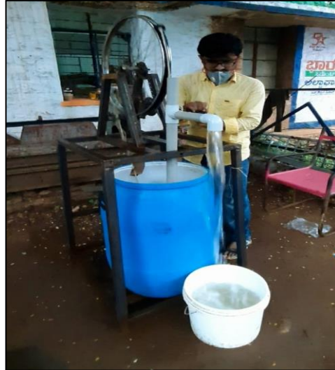
Figure 11: Hand Held Operation and Water Output of Pump
