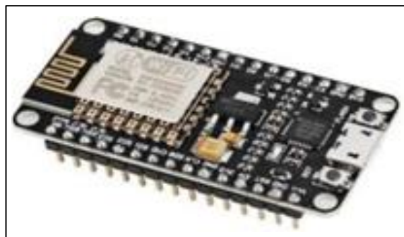
Figure 3: Node MCU (labelled)
