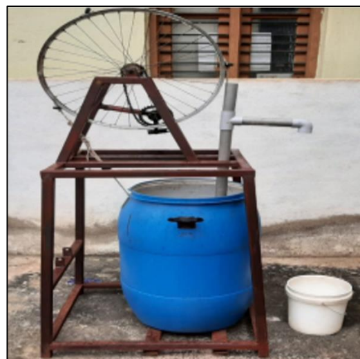
Figure 10: Assembled Model of the Water Lifting Pump
