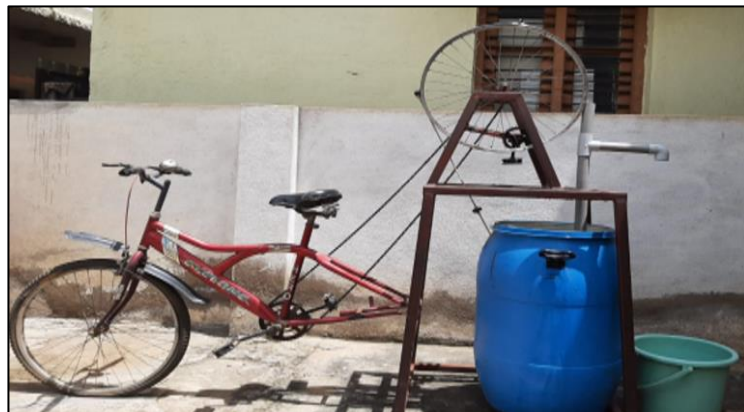
Figure 12: Side View of the Assembled Model with Peddling Mechanism
