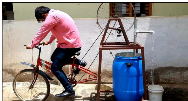
Figure 13: Peddling Operation and Water Output of Pump
