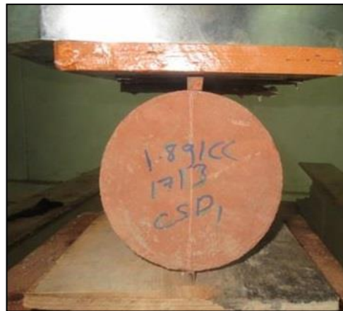
Fig 2: Split tensile strength test setup.
