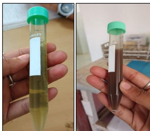
Fig 1: Change in colour shows nano particle synthesized
