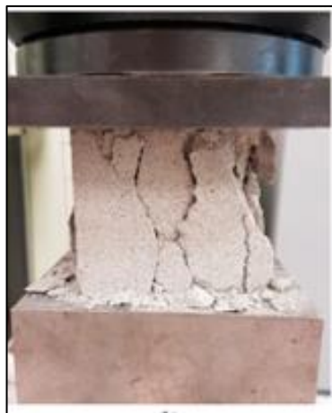
Figure 3 Failure of LDFC Cube
