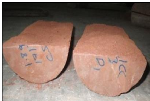
Fig 5: Typical failure pattern of cylinder specimen tested under split tension test.
