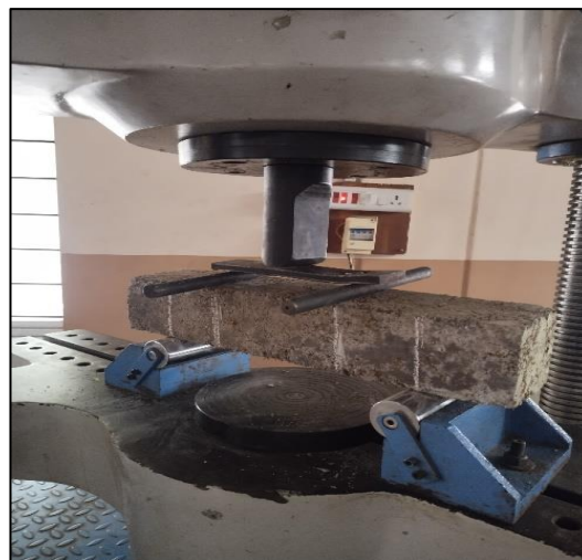
Fig.5 Flexural strength test on specimen of size 100x100x500mm
