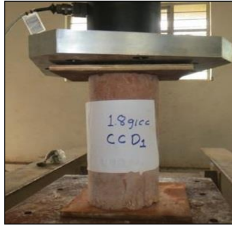
Fig 1: Compressive strength test setup.
