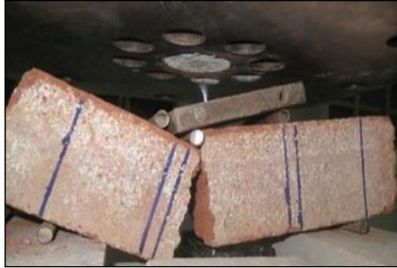
Fig 6: Typical failure pattern of beam specimen tested under flexural load.
