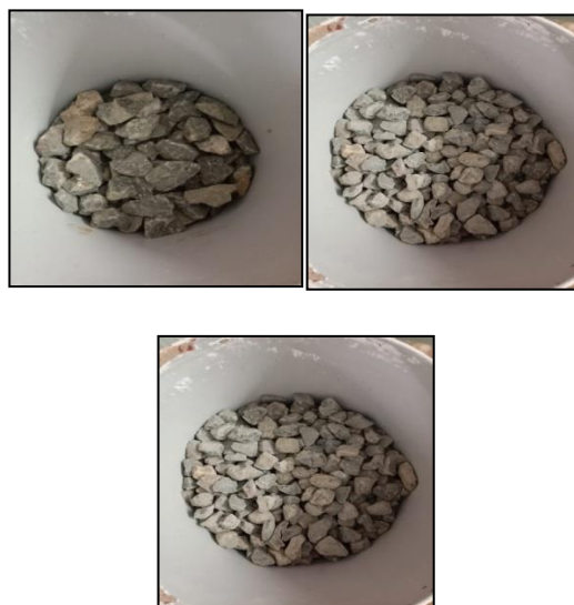
Fig 2: Aggregates of 30, 20 and 10mm passing
