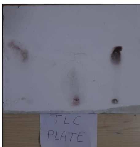
Fig 4 TLC analysis for soxhlet extract and water extract
