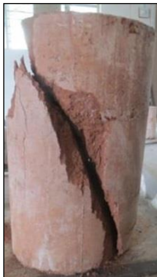
Fig 4: Typical failure pattern of cylinder specimen tested under compression.
