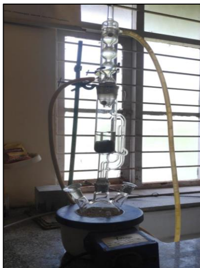
Fig. 1 Sox hlet extraction of flavonoids from Swietenia mahagoni
