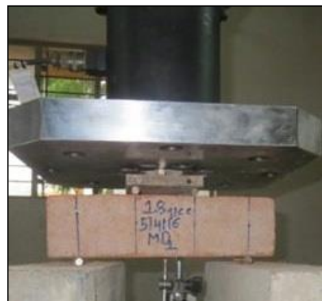
Fig 3: Flexural strength test setup.
