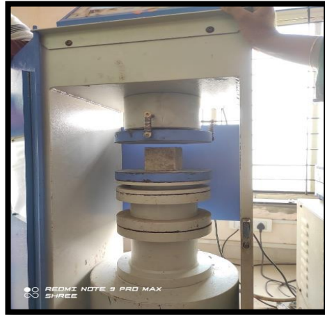
Fig.4 Compression strength test on specimen of size 75mmX75mmX75mm
