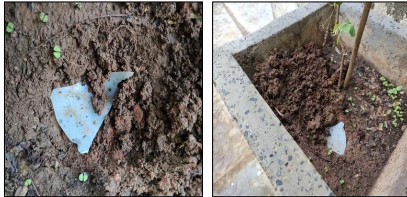
Fig. 3: Soil burial method
