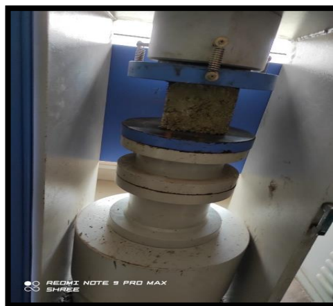
Fig.3 Compression strength test on specimen of size 100mmX100mmX100mm
