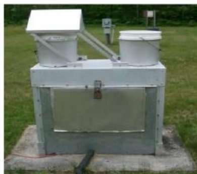
Fig. 4 Wet and Dry deposition collector (Source: NADP, n.d.).
